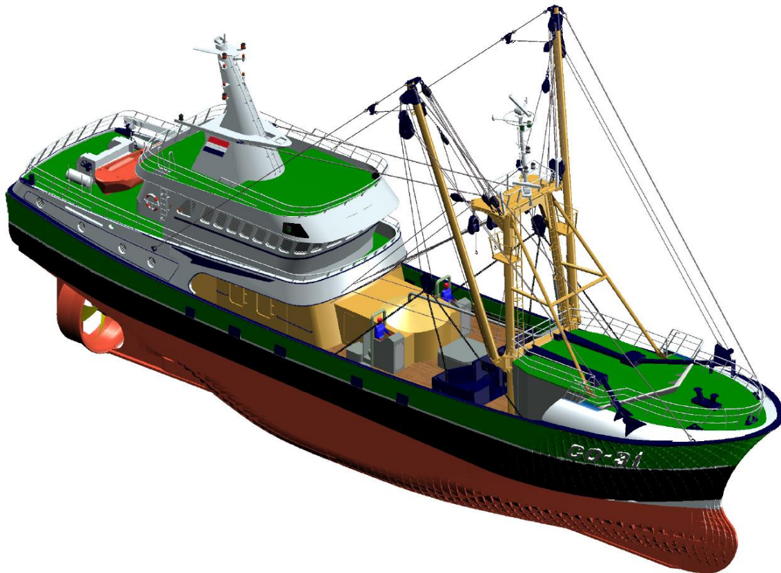
Figuur 23: Artist impression kotter GO31 met verticale LNG tankopslag (credits Van Dam - Maaskant Shipyards)
