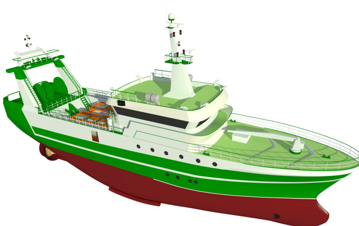
Figuur 25: Artist impression kotter PD147 met 2x20ft LNG cryocontainer (credits Ekofish Group – Koers & Vaart)
