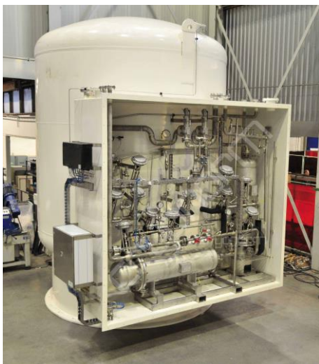
Figuur 22: Verticale LNG opslagtank en Tank Connection Space (TCS) (credits Cryonorm)
