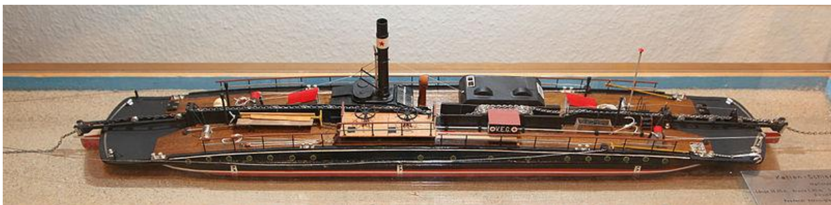
Figure 5: Model of rail towed vessel or Ketten-Schleppdampfer used on the Elbe Germany.
