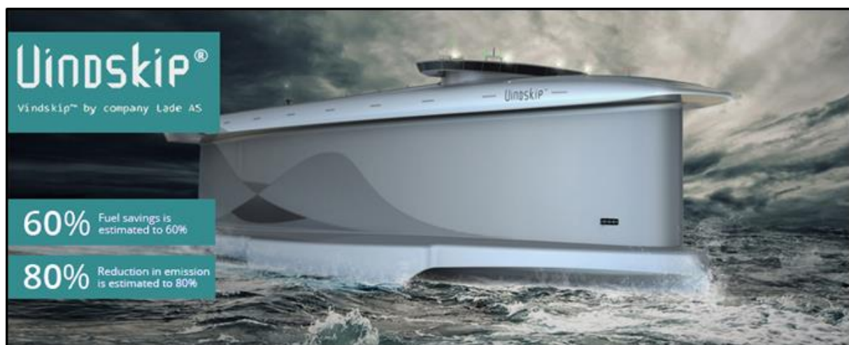
Figure 6: Vindskip concept claiming 60% energy reduction and 80% reduction of GHG emissions (Lade As, 2012)
