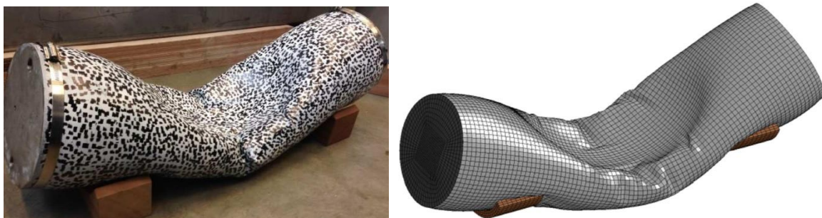
Graph 2-2-1 Model test of Impact strength of LNG fuel tanks
