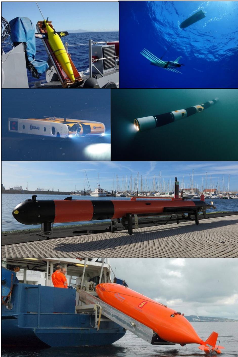
Figure 3: Collection of images showing the wide variety of AUV size and types. From left to right, from top to bottom: liquid robotics wave glider, Kongsberg sea glider, Saab Sabertooth hybrid ROV/AUV, Kongsberg Eelume AUV, oceanscan-mst man portable Light-AUV (LAUV) owned by TNO, Kongsberg (Liquid Robotics, 2019; SAAB, 2018; Eelume, 2015; OceanScan, 2018; Druglimo-Nygaard, 2014).
