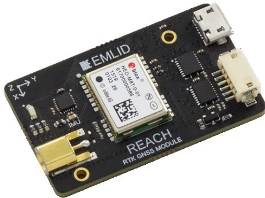
Figure 26: RTK GNSS GPS (Emelyanova, 2016)
