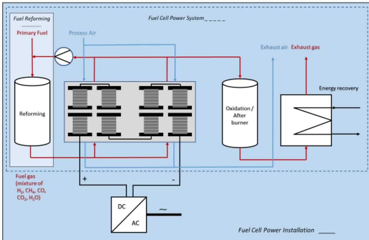
Figure 8: Generic Fuel cell Power Installation (DNV GL, 2017)
