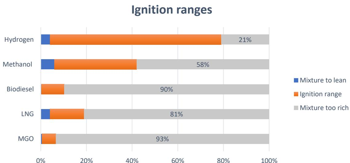
Figure 2: Ignition ranges of various alternative fuels
